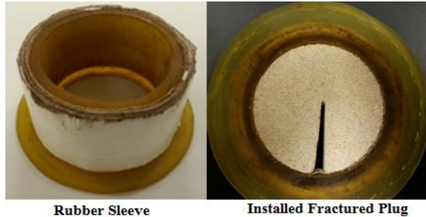
Figure 9. The developed rubber sleeve with temperature resistant adhesive tap.
